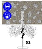
*uld be positive interaction between the steel stiles of the brush and the sides of the drilled hole.*
