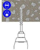
2. Select the correct Air Lance, insert to the bottom of the hole and depress the trigger for 2 seconds. The compressed air must be clean – free from water and oil – and at a minimum pressure of 90psi (6bar).
