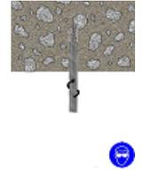
Excess resin will be expelled from the hole evenly around the steel element and there shall be no gaps between the anchor element and the wall of the drilled hole.
