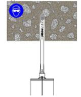
11. Select the steel anchor element ensuring it is free from oil or other contaminants, and mark with the required embedment depth. Insert the steel element into the hole using a back and forth twisting motion to ensure complete cover, until it reaches the bottom of the hole.
