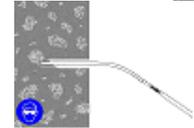
(The extension tubes may be pushed into the resin stoppers and are held in place with a coarse internal thread).
