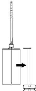
8. Extrude some resin to waste until an even-colored mixture is extruded, The cartridge is now ready for use.
