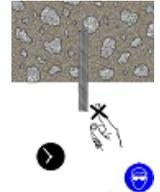
14. Position the fixture and tighten the anchor to the appropriate installation torque.
