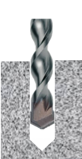
Drill correct diameter hole to correct depth
