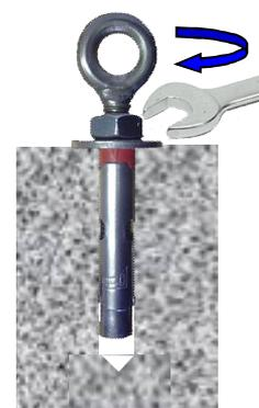
Tighten to recommended torque
