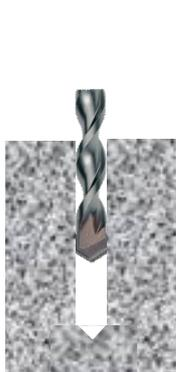
Position fixture and drill correct diameter hole to correct depth
