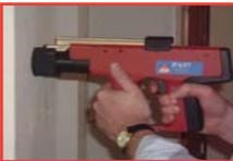
Place the tool perpendicular to the work surface and adopt a well balanced stance. Push against the tool to fully depress the fastener guide then pull the trigger.
