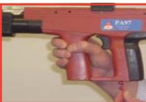
Insert the cartridge strip, leading with the end with the arrow, into the tool grip until the bottom end of the strip is flush with the tool.
