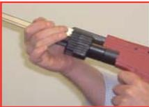
Pull back the cocking grip as far as it will go then return it to its original position. Return the cocking lever to the start position and lock the cocking grip into place.
