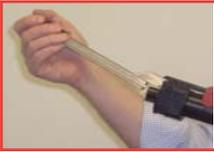
Release the cocking grip and pivot the cooking lever through 180° to the forward position.
